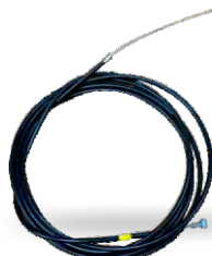
Part No.: 660353 Gasolene Control Transmission Assembly Applicability : 501 BS2 & BS3, 501 BS4,LD-cargo DSL
